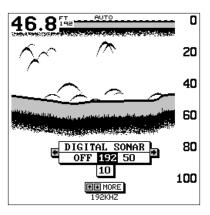
You can change the digital's frequency, if the optional SAM-50HPD is installed. To do this, or to turn it off, first press the MENU key, then press the up or down arrow keys until the "DIGITAL SONAR" menu appears. Now press the left arrow key to turn it off, or the right arrow key to select 50 kHz. Press the EXIT key to erase the menu.
